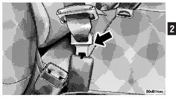
**Inserting Latch Plate**
